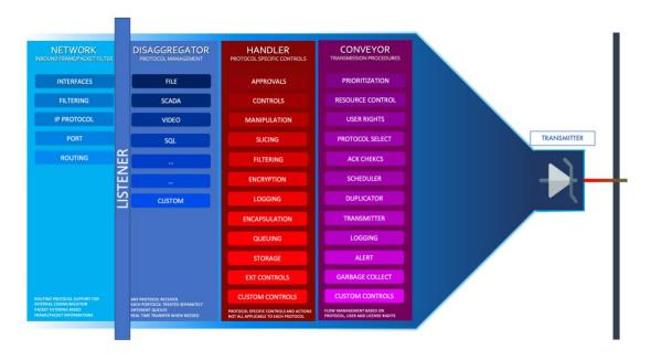
All processes defined in different layers are running separately and adding new functions and features are possible. ConnexOne limit, filter, manipulate or block any data based on application and payload.
