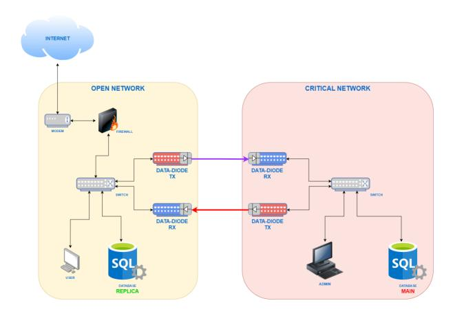
For this topology, ConnexOne devices located in the "open network" are vulnerable to cyber-attacks. Even if somehow the attacker manages to control two devices in the "open network," it is impossible for the attacker to infiltrate other ConnexOne devices (since there is no two way communication) located in the "critical network." Thus, the "critical network" is always protected.
